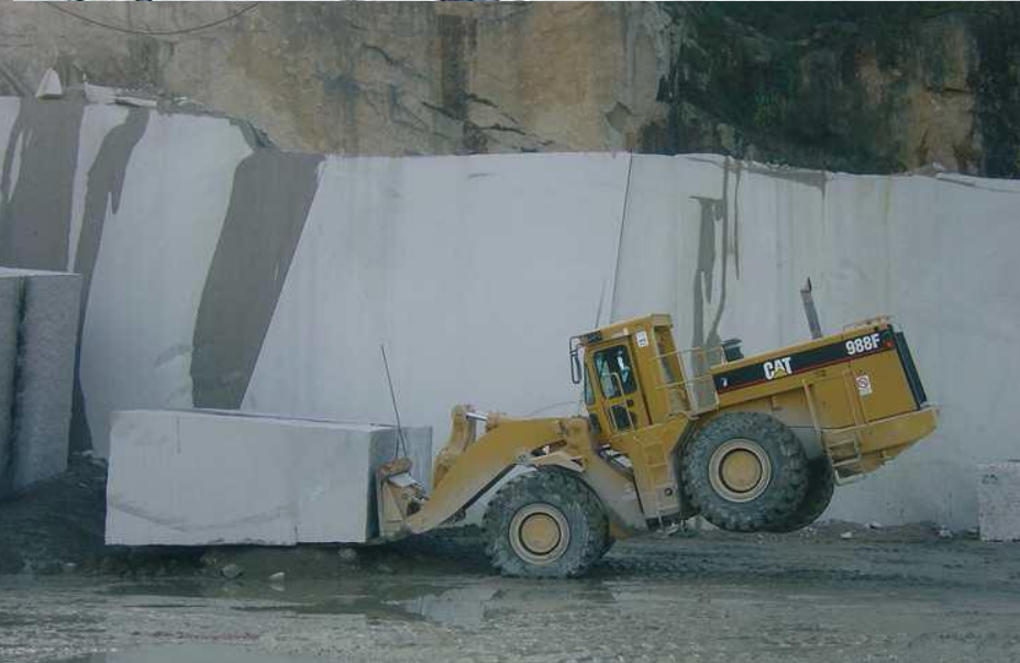
In slate, marble and granite quarries, the extracted blocks are rather large and heavy. After the cutting process, smaller pieces can be obtained, which are treated and sold for different uses
